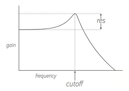
note on resonance: You may hear a slight drop in volume as the resonance is increased. This is expected because the filter is emphasizing the cutoff frequency, causing all other frequencies to drop in volume. The **output level** can be used to makeup for the volume drop.
