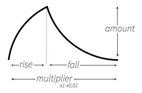
Multiplier scales both the *rise* and *fall* time from x1 to x0.01, this can be used to change the overall rate of the envelope while maintaining the ratio of *rise* and *fall* times. The *amount* control determines how much of the envelope is sent to the VCF.
