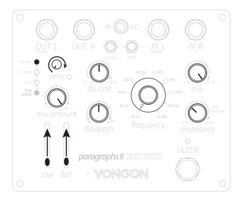
The **ENV FOLLOWER** mode uses your instrument's volume envelope to modulate the filter. The **sens** control affects how sensitive the pedal is to your instrument; the goal is to find a sweet spot where you can easily control the filter by playing your instrument.
