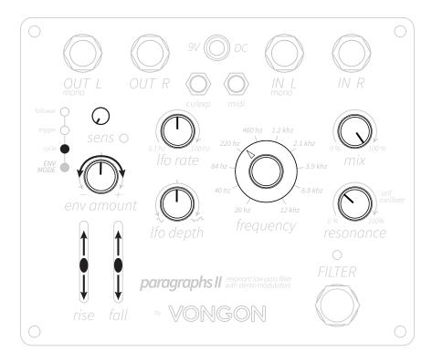
The ENV CYCLE mode will continuously loop the envelope. The *rise*, *fall*, and *env amount* controls function the same way as they do in the ENV TRIGGER mode.
