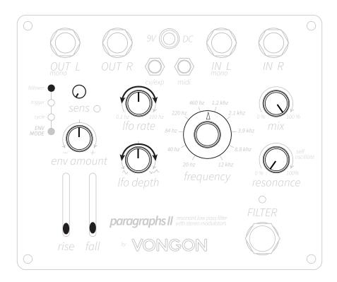
As you turn the *lfo depth* to the left, you will hear the sine wave modulation create a tremolo-style effect. If you are listening in stereo, the sound will start smoothly bouncing between the left and right speakers. If you turn the *lfo depth* to the right, you will hear the smoothed random wave modulation move your signal around the stereo space in an unpredictable way.
