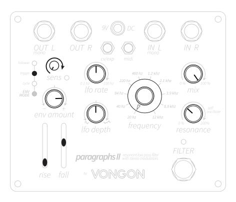
The **ENV TRIGGER** mode produces an envelope at the moment when your instrument passes a volume threshold set by the **sens** control. Using the settings shown, start to slowly increase **sens** as you play your instrument. You should be able to find a spot where you can easily trigger the envelope by playing. If the **sens** is too low, it may not trigger at all, while if it's too high, it may produce false triggers during play.
